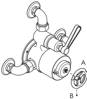
Remove the thermostatic control handwheel (A) by unscrewing set screw (B) using a 2mm hexagonal key.
