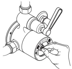
Adjust the cartridge spline whilst measuring the temperature of the water. Ideally the temperature measurement should be taken using a digital thermometer.
