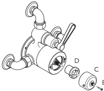
Remove the override (C) and temperature stop (D) by unscrewing and removing screw (E). Fitting handwheel (A) and set screw (B) will aid with removal of override (C).
